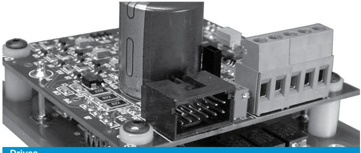
AMETEK offers variable speed brushless motor controllers in a single board with analog command input to compliment most of its brushless motors. These controllers are low voltage DC input and high current output with DSP flexibility for velocity and acceleration control.
